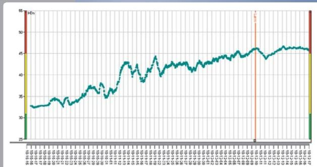
The **Shock Pulse Trend** for the slow running overhead conveyor gearbox shows a steady rise since the first readings taken. Initially the gearbox was in the green and in good condition, over the past few months the readings have risen into the red and there are signs of minor damage.
